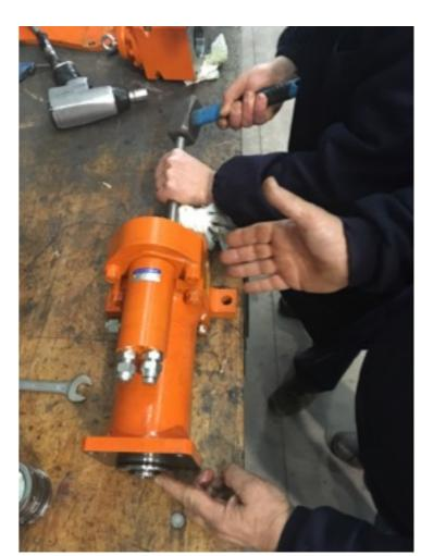
Remove the oil from the cylinder module.
