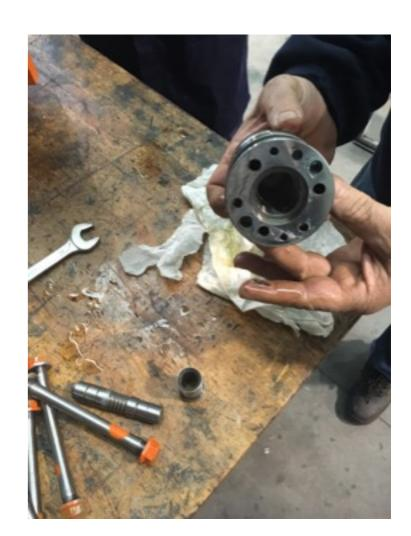
Remove the distribution box (3), eventually carefully using a soft hammer.
