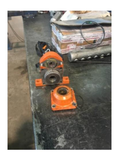
The rotation motor (12) can be disassembled removing the 2 screws (43) Remove the snap-ring (31), the seal ring (46) and the Bushings (29)
