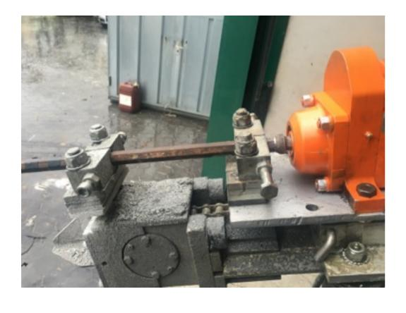
Always ensure a good alignment of the drifter / rig and the drill string:
