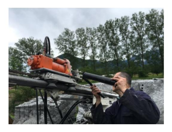
Always ensure a good greasing, hydraulic drifters work with high rotation speed and percussion frequency. Damages due to lack or improper greasing are not covered under warranty:
