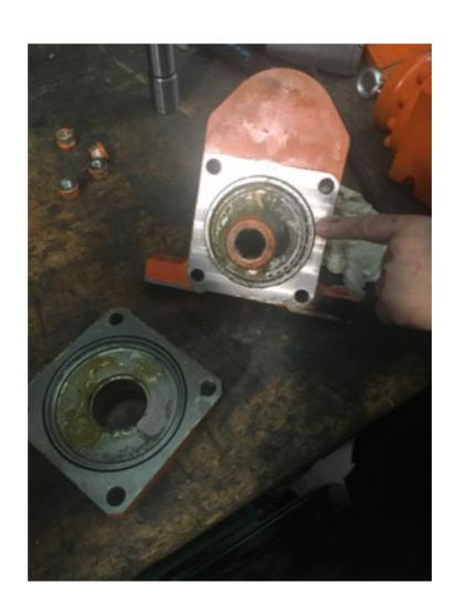
Use a soft hammer in order to remove the Hub (26) from the rotation housing (24) Carefully remove the bearing (25) and the hexagonal bushing (27) and gear (33). The Hexagonal bushing and gear can be disassembled using a press.
