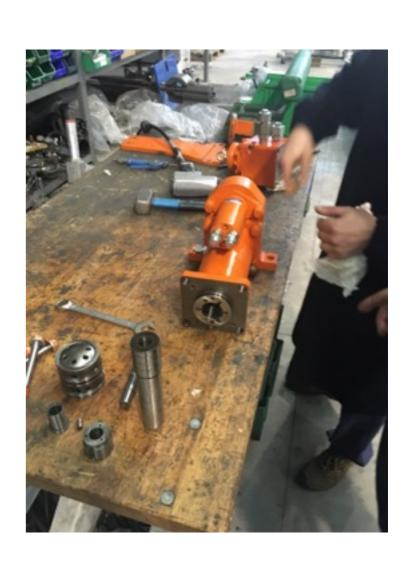
Remove the cylinder flange (8)
